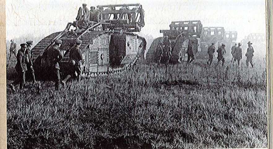
In 1916 the British became the first to use armored tanks in war. Armor protected the tanks from machine-gun fire. Caterpillar tracks allowed tanks to cross barbed-wire entanglements.
